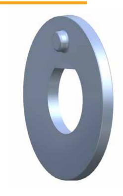
The special FKL spring washer prevents the shaft turning at the nut tightening and due to its spring properties provides 6 tons of axial clamping force.
